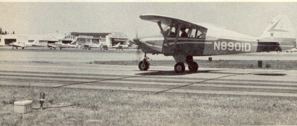
Abrams Air Traffic Counter (lower left), installed here on taxiway at a Michigan airport, reportedly gives accurate tally of a facility's operations to aid in planning and financing purposes. It works equally well on ramp or runway and on virtually all surfaces.
